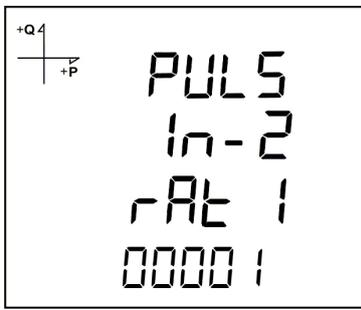
1. Press UP button while PULSE IN-2 Enable is displayed.
