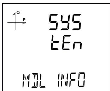
Information about the module that is installed on the device can be displayed under this menu.
