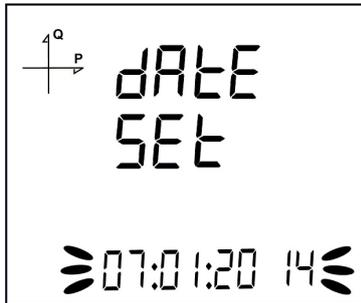
The date of the device's RTC module can be set in days, months and years.
