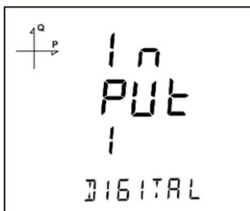
2. Generator Input: When this option is selected, the device records the energy to the generator register depending on the input state.
