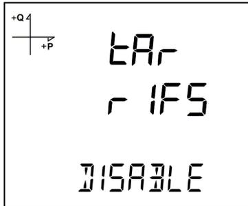
Press the SET button. If you change Disable option to Enable with UP/DOWN buttons, tariff function of the device will be activated. Press the SET button to confirm your selection.
