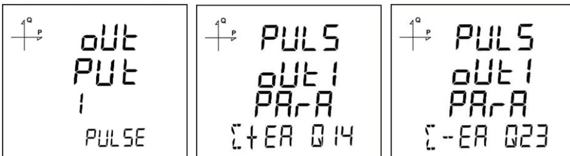
1. Press UP button while OUTPUT 1 PULSE is displayed.
