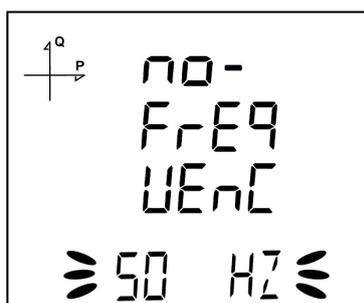
1. By using UP/DOWN buttons, select your nominal network frequency as 50 Hz or 60 Hz.
