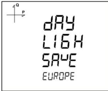
1. Press the SET button while Clock DST Mode screen is displayed.
