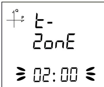
1. By using UP/DOWN buttons, you can select the time zone information about the device location between -12:00 and +12:00 in 30 minute intervals.
