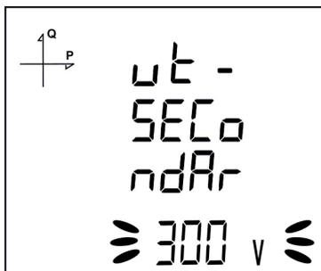
1. Enter the secondary value of your VT by using SET and UP/DOWN buttons.
