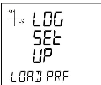
1. Press the SET button while Log Setup-Load Profile is displayed.
