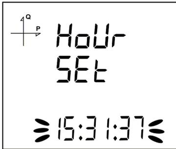
1. Enter the time by using SET and UP/DOWN buttons.
