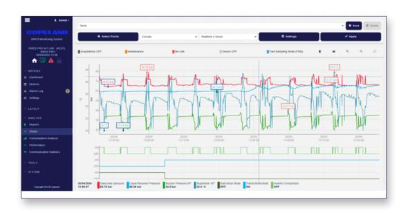
The advanced alarm management system is one of the strengths of the XWEB PRO family. It allows for alarm notification emails that embed the enhanced data analysis mentioned earlier, thereby facilitating the remote identification of malfunction reasons by the technical support staff as soon as they occur.
