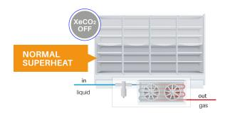
XeCO<sub>2</sub> has the capability to reduce the superheat set-point of the medium-temperature line cabinets, while also preventing overfeeding of evaporators and enhancing the cooling capacity of the system, thereby ensuring maximum system security.
